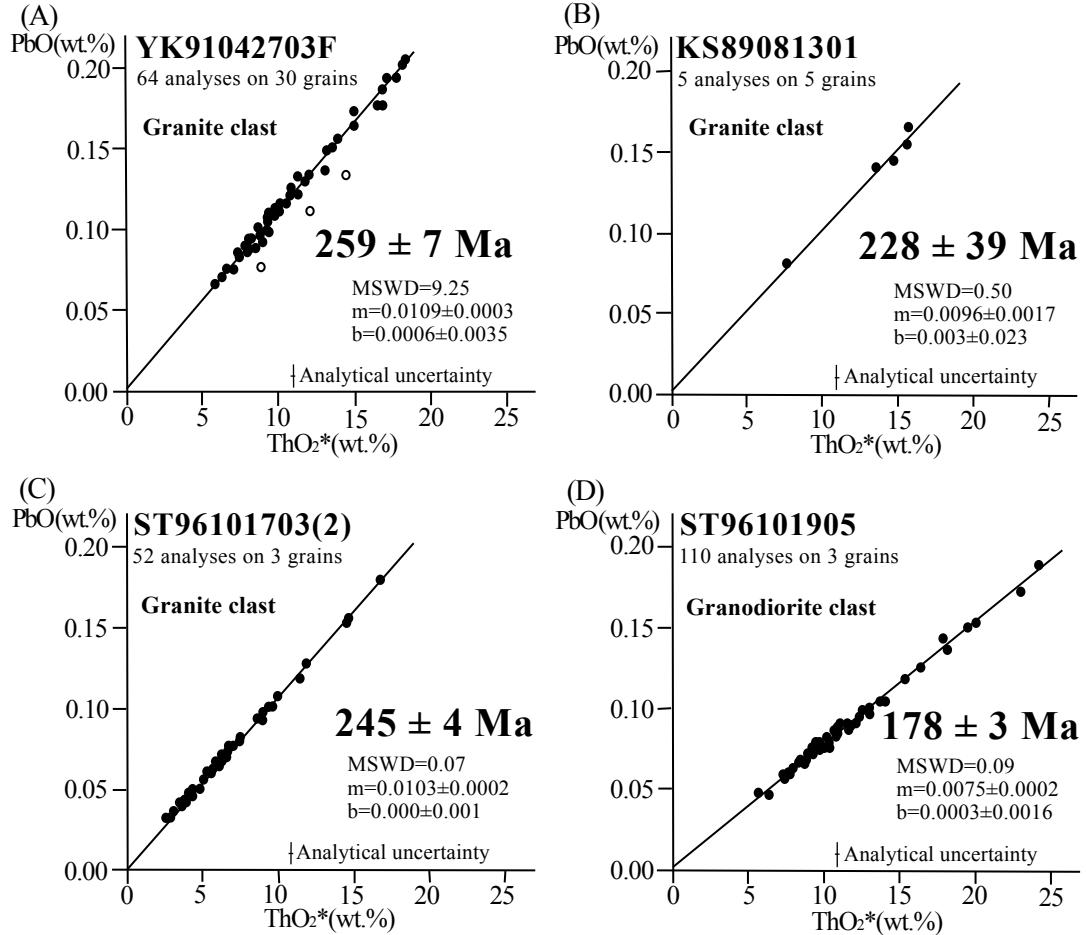
Fig. 5. Plots of PbO vs. ThO<sub>2</sub>\* for monazite from the granitoid clasts. (A): Sample YK91042703F (granite clast). (B): Sample KS89081301 (granite clast). (C): Sample ST96101703(2) (granite clast). (D): Sample ST96101905 (granitoid clast). Error bars and quoted error are of  $2\sigma$ . MSWD: Mean Square Weighted Deviates. Open circles in (A) show data from grain rim. ThO<sub>2</sub>\*: measured ThO<sub>2</sub> plus ThO<sub>2</sub> equivalent of the measured UO<sub>2</sub>.
